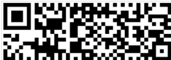
Like with QR Code, rMQR Code employs Reed-Solomon error control coding to detect and correct errors if the rMQR barcode is dirty or damaged. rMQR Code uses variable error correction levels and can handle all types of data. rMQR Code is capable of storing up to 361 numeric characters and 219 alpha-numeric.
