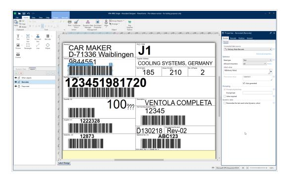
Figure 2: Using layers during label design
