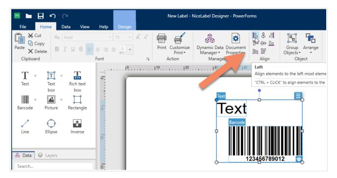
Figure 8: Alignment commands available directly in the ribbon
